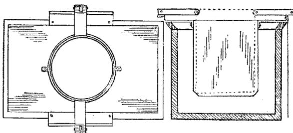
FIGS. 28, 29.—PLUNGE TANK, IN PLAN AND SECTION.
