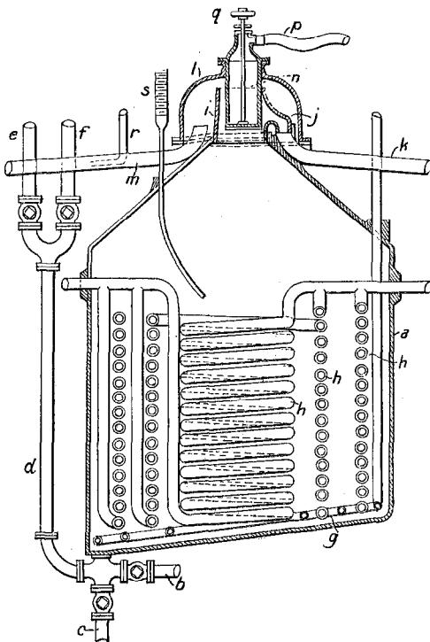
FIG. 7.—NATHAN'S NITRATOR FOR NITRO-GLYCERINE. (a) Nitrating Vessel; (b) to Separating Vessel; (c) to Drowning Tank; (e) Nitrating Acids enter (f) to the Waste Acids; (g) Coils for Compressed Air; (h) Pipes for Cooling Water; (i) Glass Cylinder; (j) Outlet to k; (k) leading to Prewash Tank; (l) Glass Dome; (m) Pipe to lead off for Escape of Fumes; (n) Vessel; ( $\rho$ ) Pipe conveying Glycerine; (q) Knob to turn off Glycerine; (r) Compressed Air Jet; (s) Thermometer.
