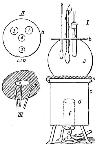
FIG. 46.—HEAT TEST APPARATUS.
