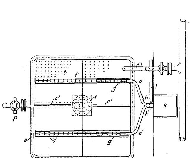
FIG. 21.—PLAN OF THOMSON'S APPARATUS. *a*, Tank; *b*, False Bottom; *c*, Ribs; *e*, Grid; *f*, Troughs; *g*, Aprons; *h* and *h'*, Pipes to Troughs *f*; *k*, Sulphuric Acid Tank; *m*, Pipe to Nitrating Acids Tank; *o*, Perforations of Troughs; *p*, Cock to remove Acid.
