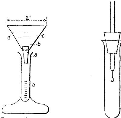
FIG. 47.—APPARATUS FOR SEPARATING THE NITRO-GLYCERINE FROM DYNAMITE.
