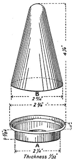
FIG. 40.—MARSHALL'S APPARATUS FOR MOISTURE IN CORDITE.
