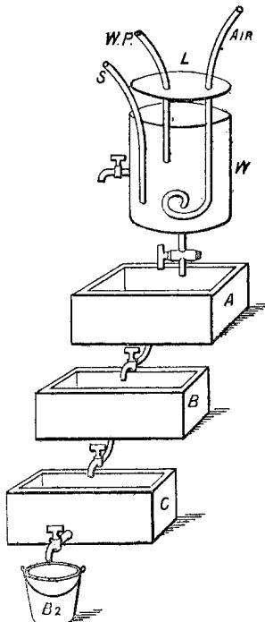
FIG. 9.—**FILTERING AND WASHING PLANT.** *W*, Lead Washing Tank; *WP*, Water Pipe; *L*, Lid; *S*, Nitro-glycerine from Separator; *A*, *B*, *C*, Filtering Tanks; *B<sub>2</sub>*, Indiarubber Bucket.
