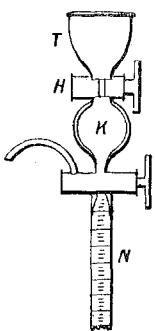
F. M. Horn (*Zeitschrift für angewandte Chemie*, 1892, p. 358) has devised a form of nitrometer (Fig. 43) which he has found especially useful in the examination of smokeless powders. The tap H is provided with a wide bore through which a
