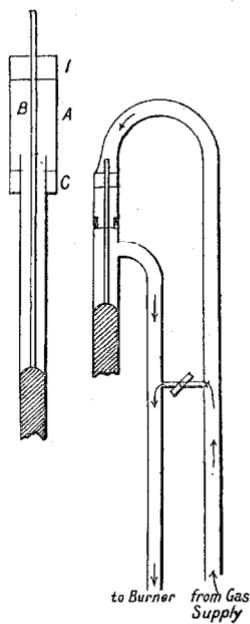
FIG. 50.—PAGE'S GAS REGULATOR, SHOWING
