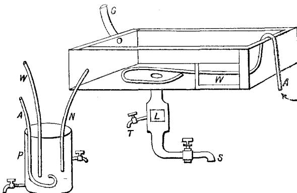
FIG. 8.—SEPARATOR. *A*, Compressed Air Pipes; *G*, Nitro-glycerine enters from Nitrator; *N*, Nitro-glycerine to *P*; *L*, Lantern Window; *W*, Window in Side; *S*, Waste Acids to Secondary Separator; *T*, Tap to remove last traces of Nitro-glycerine; *P*, Lead Washing Tank; *A*, Compressed Air; *W*, Water Pipe; *N*, Nitro-glycerine from Separator.
