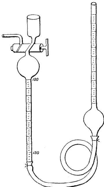
FIG. 41.—ORDINARY FORM OF LUNGE NITROMETER.
