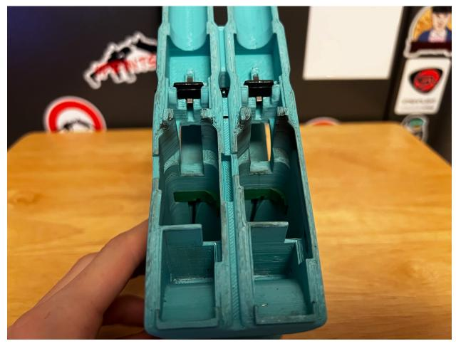
If for some reason your magazine catch doesn't move freely even after ensuring all supports are removed (and you are sure you followed the print settings in the readme), you can use a rat-tailed file and a screwdriver to remove a little material from the slot until the magazine catch moves freely (this shouldn't be required and is a sign that your settings are wrong/printer isn't dialed in).
