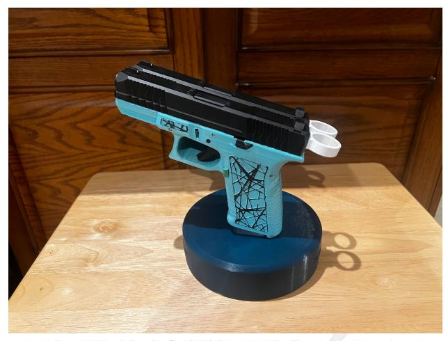
At this point, rack the slides, dry fire, hold the triggers down, rack the slides, release the triggers, dry fire again. The slides should be fairly easy to rack. You can use a little grease or oil on the rails to allow things to move a little more smoothly if things are tight. After a little test firing everything should break in nicely. The next section will guide you through some basic troubleshooting.
