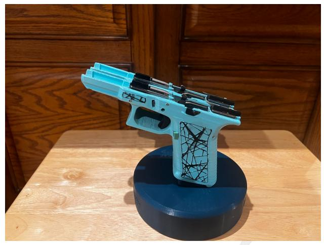
Push the pin all the way. Before you push it past the slide stops, make sure the springs on the slide stops are underneath the little (top) pin in the locking blocks and not over the top of them. The big (bottom) pin should feel like it "clicks" into place once you've fully inserted it.
