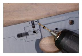
Using a 1.5mm drill bit, chase out the outer-most face of the bolt-catch cross-pin geometry.
