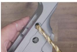
Using a 6.5mm drill bit, chase out the takedown pin geometry on the receiver.
