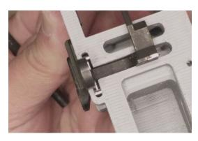
Use the flat end of the starter punch to seat the pins flush into the receiver.
