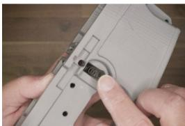
Place the magazine catch spring and magazine catch button into the lower receiver.
