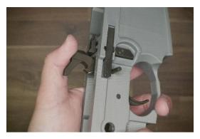
Insert the hammer assembly and pin it in place.
