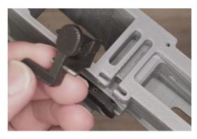
Place the bolt catch into the bolt catch channel.
