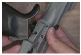
Insert the takedown detent and fire selector detent.
