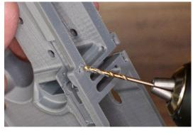
Using a 1.5mm drill bit, chase out the top-most face of the ambidextrous bolt release pin geometry.
