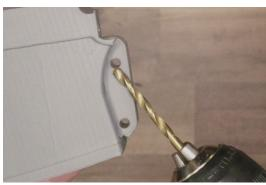
Using a 4.0mm drill bit, chase out the takedown offset screw geometry on the receiver.
