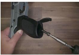
Screw in the grip screw to the receiver.
