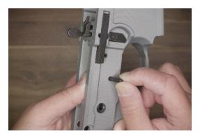
Insert the trigger assembly and pin it in place.
