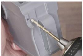
Using a 2.5mm drill bit, chase out the front takedown spring channel.
