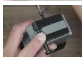
Pivot down the other takedown offset. Secure and tighten the takedown offset screw.
