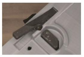
Ensure the ambidextrous control is seated completely to the front of the receiver.
