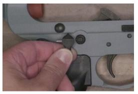
Place the ambidextrous fire-control onto the fire-control selector.
