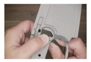
Spin the magazine release to secure it in place with the magazine release button.
