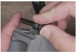
Using the takedown pin, pivot the takedown offset on top of the detent into the spring in the channel.
