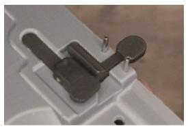
Insert the bolt catch cross pins into the receiver.
