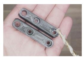
Using a 4.0mm drill bit, chase out the takedown offset screw geometry on the takedown offsets themselves.
