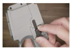
Remove the magazine catch geometry of all debris. Fit and insert the magazine catch.
