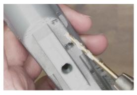
Using a 2.5mm drill bit, chase out the rear takedown spring channel.
