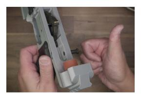
Briefly check the rear takedown pin and fire-selector. Both should move smoothly, and with a tactile feeling of the detent engaging.
