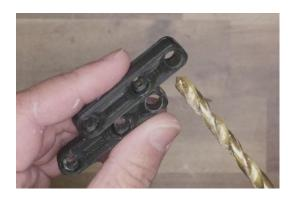
Using a 6.5mm drill bit, chase out the takedown pin geometry on the takedown offsets.
