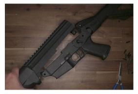
Attach the upper receiver to the lower receiver, starting with the front-most takedown pin.
