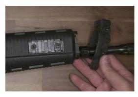
Attach the false gas block/shroud retainer to the barrel. Press it against the shroud.
