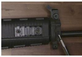
Tighten the false gas block.
