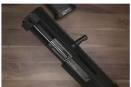
Fully insert the bolt into the receiver.
