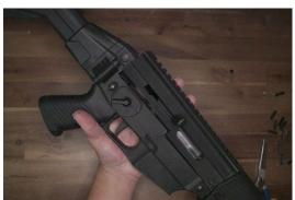
Collapse the receivers together, and close the rear takedown pin.
