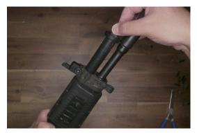
Insert the false adjuster into the false gas-block.
