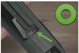
Ensure the breach face is flush to the internal breach face of the receiver.
