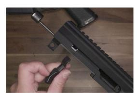
Insert the bolt assembly partially into the upper. With the notch for the charging handle visible in the rear of the receiver, insert the charging handle.
